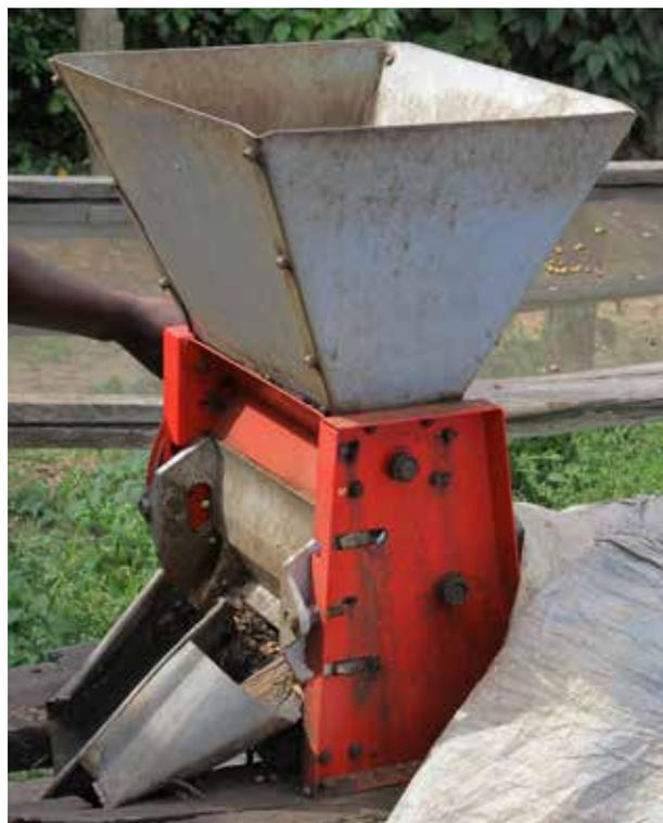
**Figure 67.** A manual pulper for removing the skins off fresh cherries
